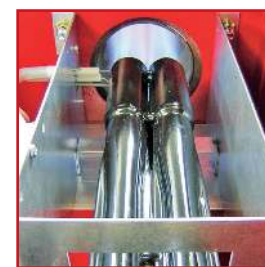
Bruciatore multiventuri in vena d'aria Air-stream burner with multi-venturi tubes
